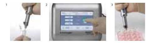
Figure 9.7. Simple 3-step transfection procedure. 1. Load mix of harvested cells and molecules to be delivered (e.g., DNA, RNA, protein) into the Neon<sup>™</sup> system pipette tip. 2. Plug the pipette into position in the Neon<sup>™</sup> transfection device, select your protocol, and press Start. 3. Unplug the pipette and transfer your transfected cells into a tissue culture vessel.
