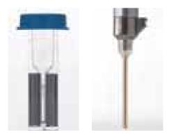
Figure 9.6. Standard electroporation cuvette compared to Neon™ system pipette tip. The design of the electrode in the pipette has been shown to produce a more uniform electric field. The result is less toxicity to the cells and higher transfection efficiencies.
