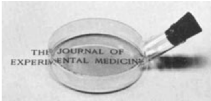
Figure 1. One of Carrel's D-flasks which were manufactured from PYREX glass.
